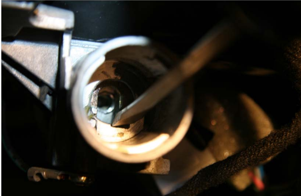
Using a Small Screwdriver to Press Down the Steering Wheel Locking Tab
